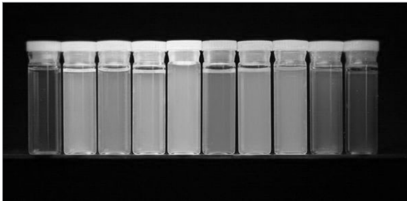
Quantum dots can emit visible light of any wavelength, leading to these multi-colored solutions of colloidal quantum dots.
